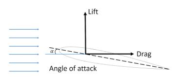
Figure 2. lift and drag components of airfoil
