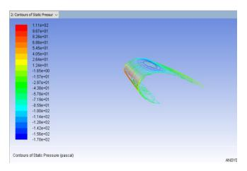
**Contour 2.** Static pressure variation for profile EPPLER863 with one fourth trailing edge removed
