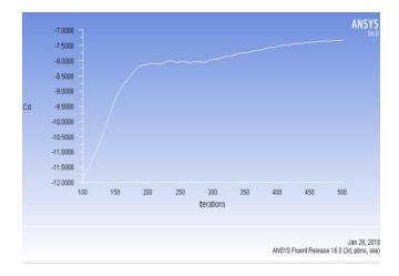
Graph 3. Iterations of drag coefficient for profile Lenz2
