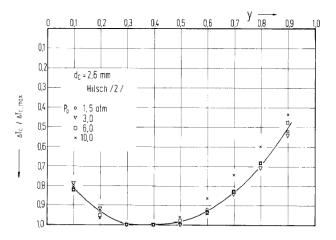
Fig -7: Similarity relation, equation (25), compared with experimental data of Hilsch <sup>[2]</sup>[8].
