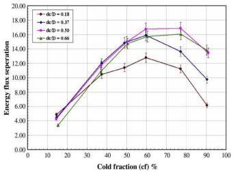
**Fig -5**: The effect of orifice diameter on the energy flux separation efficiency (mi = 0.45 kg/min). Error bars in the graph indicate 5% of experimental error [5].
