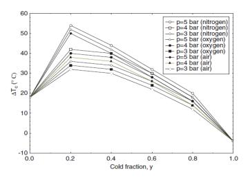
Fig-4: Comparison of the thermal performance of different gases.[4]
