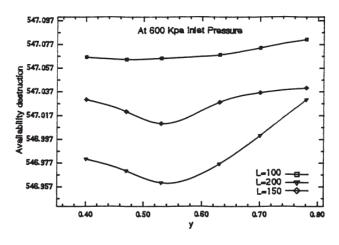
Fig -6: Variations of Exergy destruction versus tube length[7].
