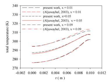
**Fig -3:** Comparison of the variation of total temperature versus radial distance at different axial locations from the inlet on the plane crossing longitudinally vortex tube and including its axis between Aljuwayhel work and present axisymmetric work.[3]
