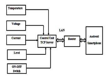
Fig -4.1: Block Diagram of Smart Control Generator by using Android Application
