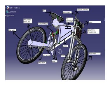
(FIG.2.2.1 SHOWS CONSTRUCTION OF "DEMON")
