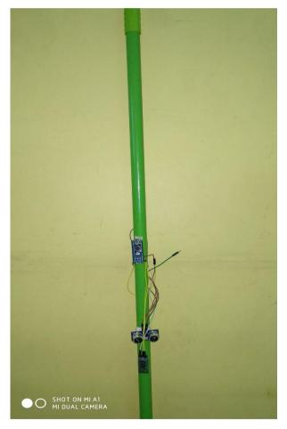
This system presents a concept to provide a smart electronic aid for blind people. The system is intended to provide overall measures artificial vision and object detection, real time assistance via global positioning system (GPS). The aim of the overall system is to provide a low cost and efficient navigation aid for blind which gives a sense of artificial vision by providing information about the environmental scenario of objects around them.[2]
