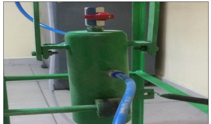
Fig -7: Actual view of mixing chamber
