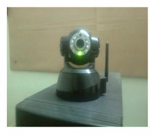
An internet protocol camera or we can say an IP camera is used as a camera for a digital video which is commonly used for surveillance or for security purpose, and which, unlike analog closed circuit television (CCTV) cameras, which can send and also receive data via a computer network and also from the internet.
