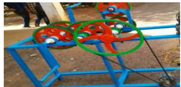
Fig - 3.4: Complete system of electricity generation.
