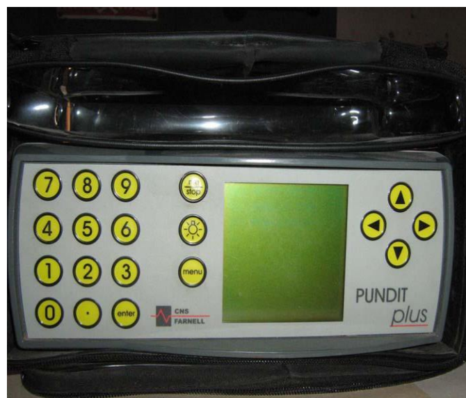
Figure 4:- USPV tester used in the Project
