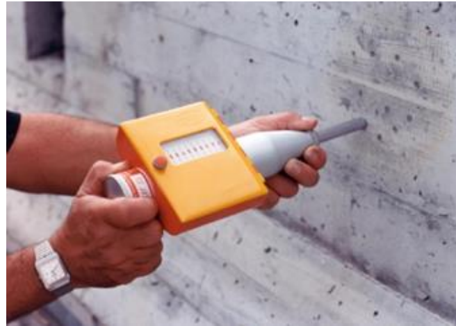
Figure 3:- Rebound Hammer Testing of a Specimen
