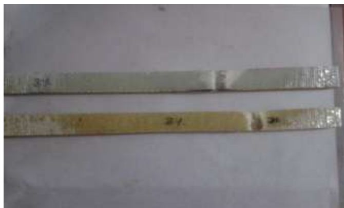
Fig.7: Failure of test specimens under tensile loading (both woven and chopped type with 3% filler)
