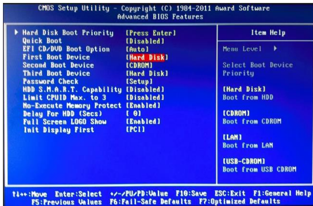
Figure: Hard disk is selected as first boot device at BIOS level.
