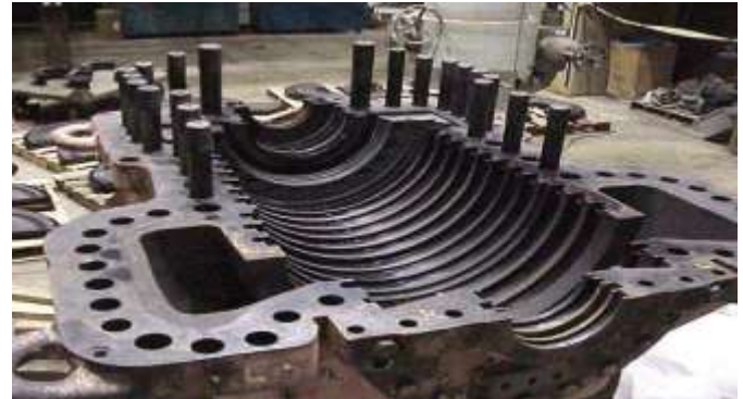
Fig -1.2 : Steam turbine casing
