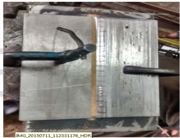
Fig -1: SS 304L plates with clamping for flat welding position.
