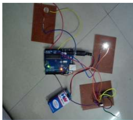
Fig - 7: Transmitter circuit with LED, LDR and Arduino
