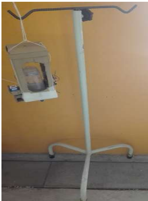
Fig - 9: The entire setup of the intravenous fluid level indicator mounted on the stand
