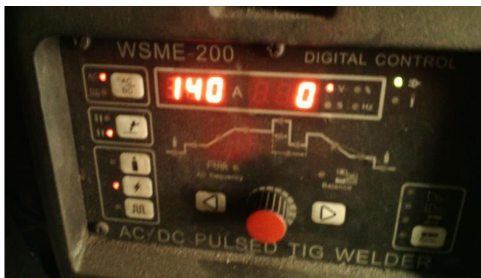
Figure 3: AC welding machine showing current as 140 Ampere
