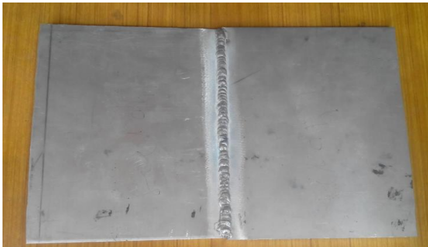
Figure 5: Welding Plate after TIG Welding at the value of current as 140 ampere
