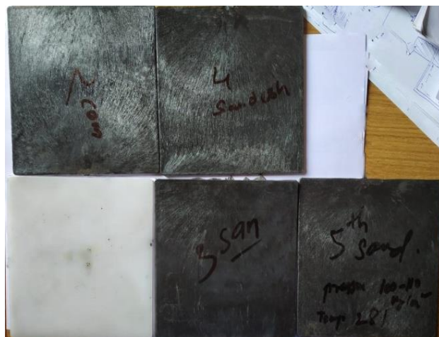
Figure 3.4 Specimen prepared by injection molding
