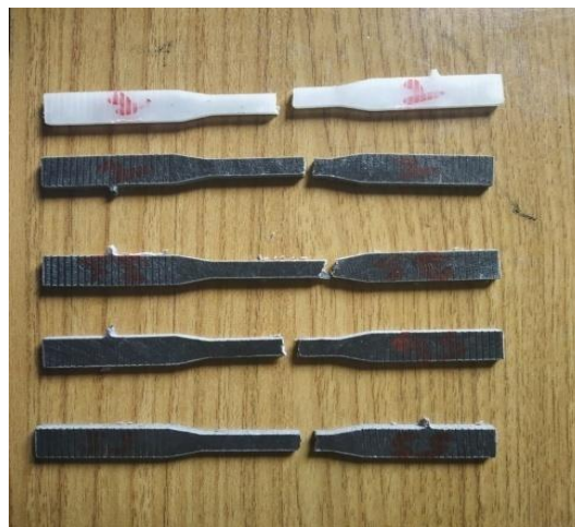
Figure 4.2 Specimen after tensile test
