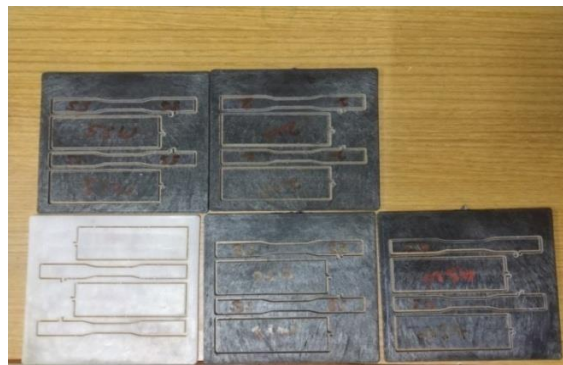
Figure 3.5 Cutting of Specimen as Per ASTM Standard
