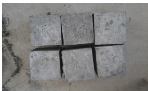
Figure 2 Casting of cubes
