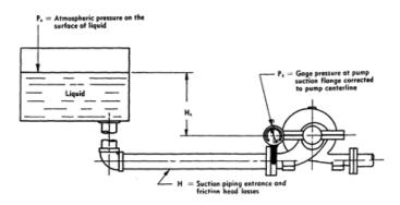
Fig 1.1 Open tank with liquid level above pump centerline.
