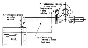
Fig.1.2 Open tank with liquid level below pump centerline
