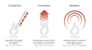
Fig-3: Conduction, Convection and Radiation [6]
