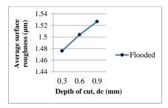
Figure 3: Effect of depth of cut on surface roughness
