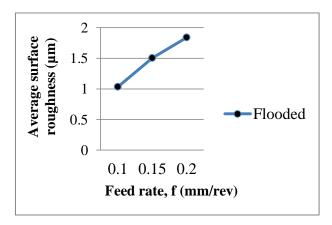
Figure 2: Effect of cutting feed on surface roughness
