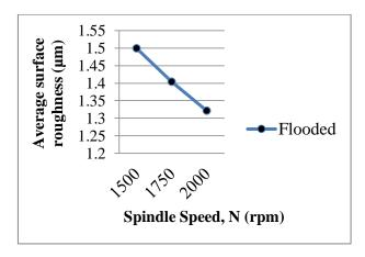
Figure 1: Effect of Spindle Speed on surface roughness
