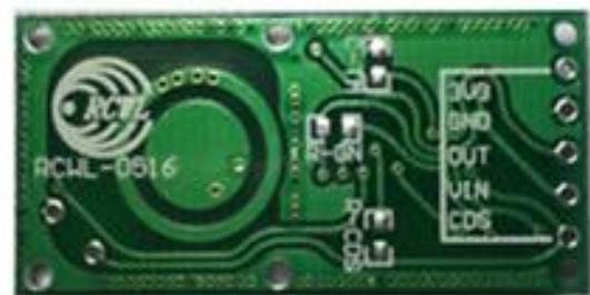
Figure 4: RCWL-0516 Human body Induction Switch Module design
