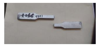
Fig.4: Specimen after subjected to tensile test
