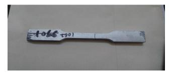
Fig.3: Specimen before subjecting to tensile test
