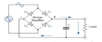
Fig 3: Bridge Wave Rectifier
