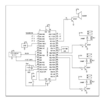
Fig2: Circuit diagram of detection and protection circuitry
