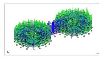
Fig -4: Live load diagram
