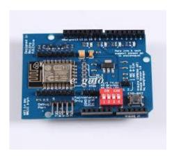
The ESP8266 is a low-cost Wi-Fi microchip with full TCP/IP stack and microcontroller capability produced by Shanghai-based Chinese manufacturer, Espressif Systems. The ESP8266 WiFi Module is a self-contained SOC with integrated TCP/IP protocol stack that can give any microcontroller access to your WiFi network. The ESP8266 is capable of either hosting an application or offloading all Wi-Fi networking functions from another application
