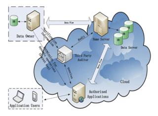
Figure 2: Audit System Architecture for Cloud Computing
