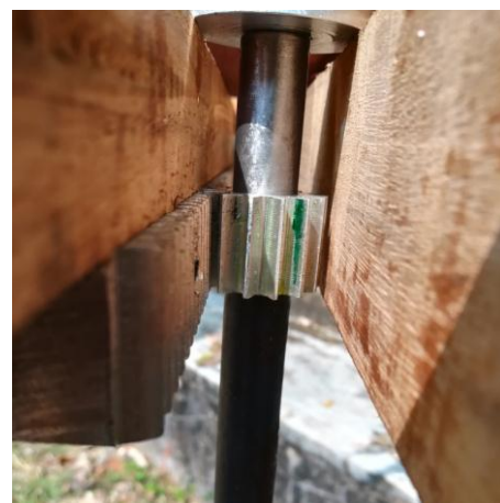
Fig - 4. Rack and Pinion Arrangement
