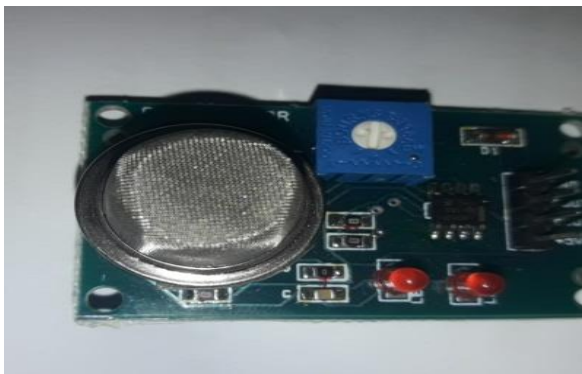
FIG:9 Gas sensor
