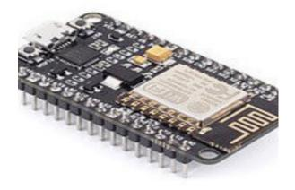
Fig -4.2a: Node MCU (ESP8266)
