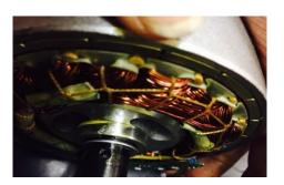
2) Shaft with copper winding attached basically configuration to rotate the shaft using electrical energy to obtain some mechanical work.
