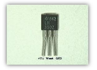
FIGURE 1: LM35 TEMPERATURE SENSOR
