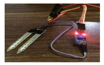
FIGURE 3: SOIL MOISTURE SENSOR YL38
