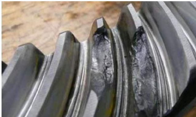
Fig 1- Interference due to improper meshing [3]
