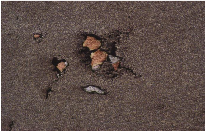
Figure: 5. Clustering of particulates Al-15%Cu composite, 100x [31]
