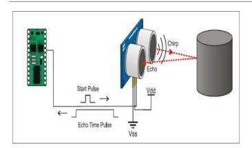
Fig-2: Ultrasonic Sensor
