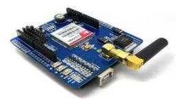
Fig-3: GSM Module
