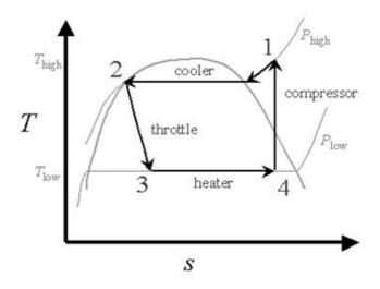
Fig -2: T-S diagram of vapour compression cycle
