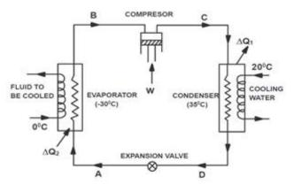
Fig -1: Vapour Compression Cycle
