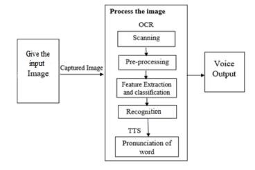
Fig -2: Flow of Process
