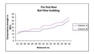
Fig.9 Rebound hammers result for first floor Bal Vihar building
