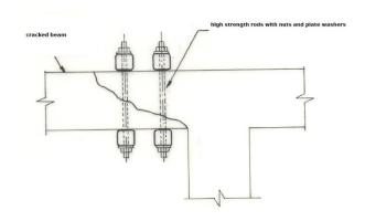
Fig.5 Cracked beams
