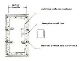
Fig.11 strengthening of the existing colum
