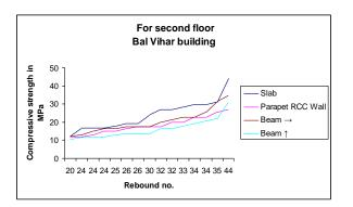
Fig. 10 Rebound hammers results for second floor Bal Vihar building
