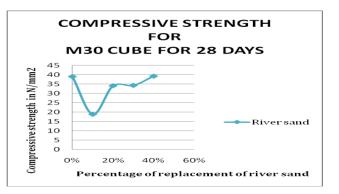
From table it was found that the graded sand replaced with River sand has shown higher value of compressive strength. The maximum increase in percentage of compressive strength was found to be 85.64% for both graded River in M20 concrete, 83.56% for both graded River in M25 grade concrete, 80.87% for both graded River sand in M30 grade concrete. Therefore the offshore sand can be effectively utilized in concrete with partial replacement of River sand.
