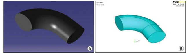
3D Model created in CATIA 3D Model imported in ANSYS
