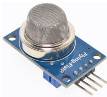
Fig -8: MQ-6 Gas Sensor
