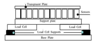
The top layer is a transparent plate to protect the sensors from getting damaged. The plate has to be transparent in order to allow the light to pass through it.
