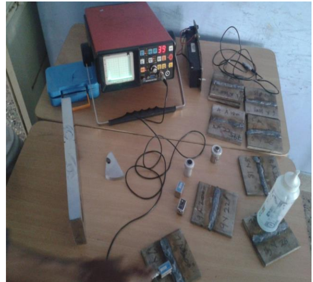
Fig 5 experimental setup of ultrasonic testing
