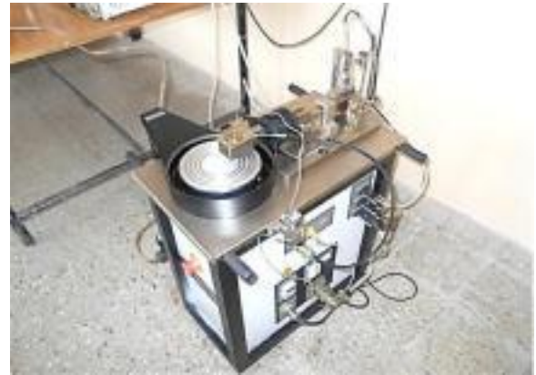
Fig4: Pin- on- disc tribometer
