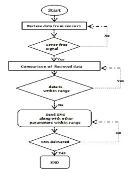
Figure 4. Flow chart of alert system
