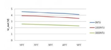
Figure 3. Voltage-Temperature characteristic
