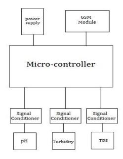
Figure 1. Design of System
