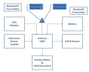
Fig -3 : Functional Block Diagram of Automated Speed Control of Auto motives
