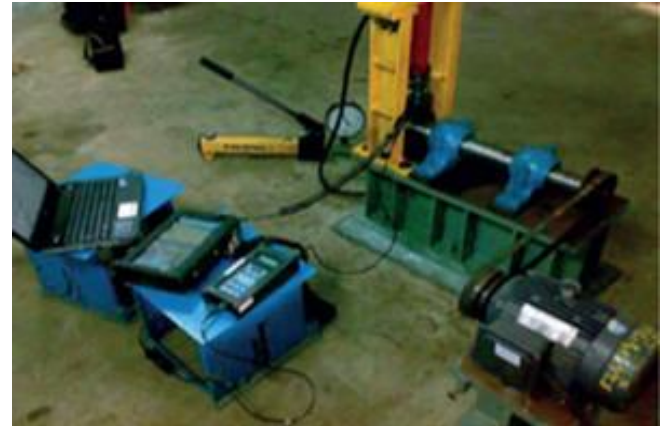
Figure 4. Bearing Test Rig with Probes
