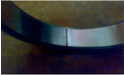
Figure 6. Outer race seeded line defect (0.5 mm width)
