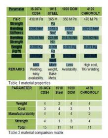
From the above table it is clear that the material to be selected is 3074 CDS4 with the help of proper optimization.
