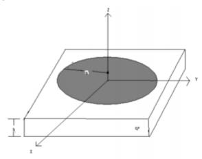
Fig1 Geometry of circular patch antenna
