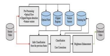
**Fig - 2**: System architecture of source LDR to enhanced HDR.
