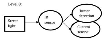
Figure 1: This shows how the street light works when human begins were present in the street.
