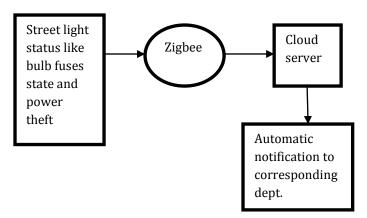
Figure 2: This shows how the notification is generated over the zigbee technology.
